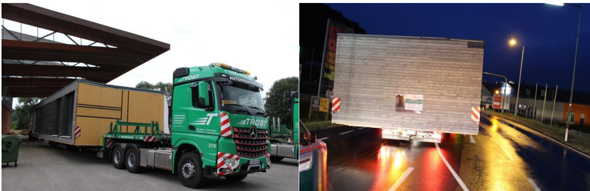
Picture 3+4 Transporting the 5.5 meter-wide GreenFlexStudioBoxes
